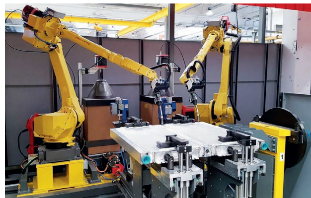
After the brazing process of the core element in Hydac's coolers, the components pass through a press to eliminate deformations and are then prepared for welding, an operation carried out with dual-arm welding robots for the largest elements.
